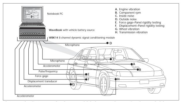
The WaveBook and WBK14 signal conditioning module both convienently operate from the 12V vehicle battery, so test engineers can gather much of the data on actual road trips. Panel rigidity tests, on the other hand, are typically conducted in the lab.
